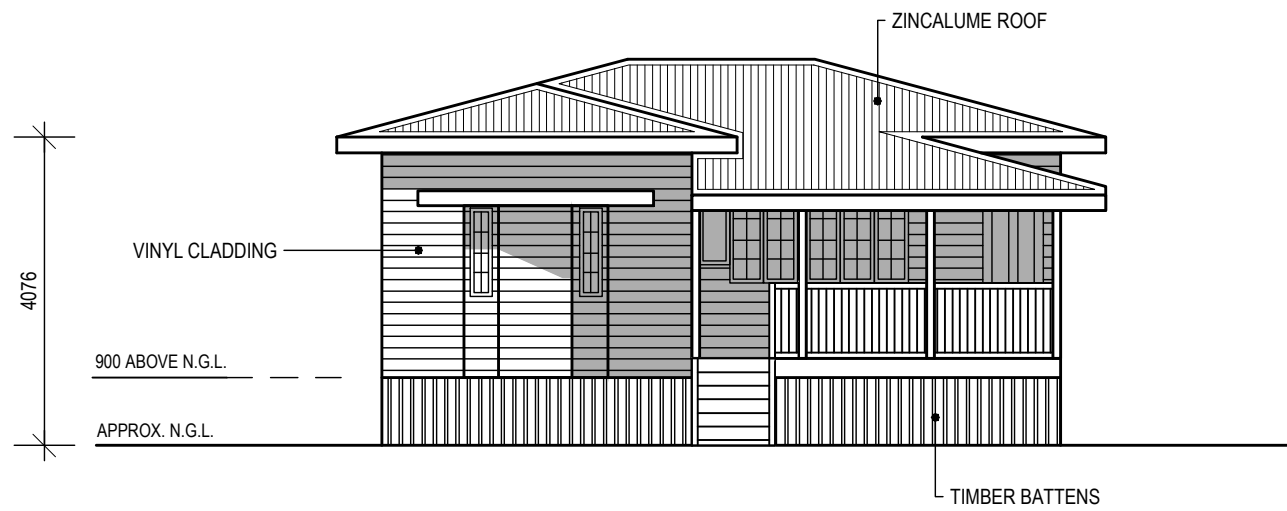
NORTH ELEVATION (FRONT)
