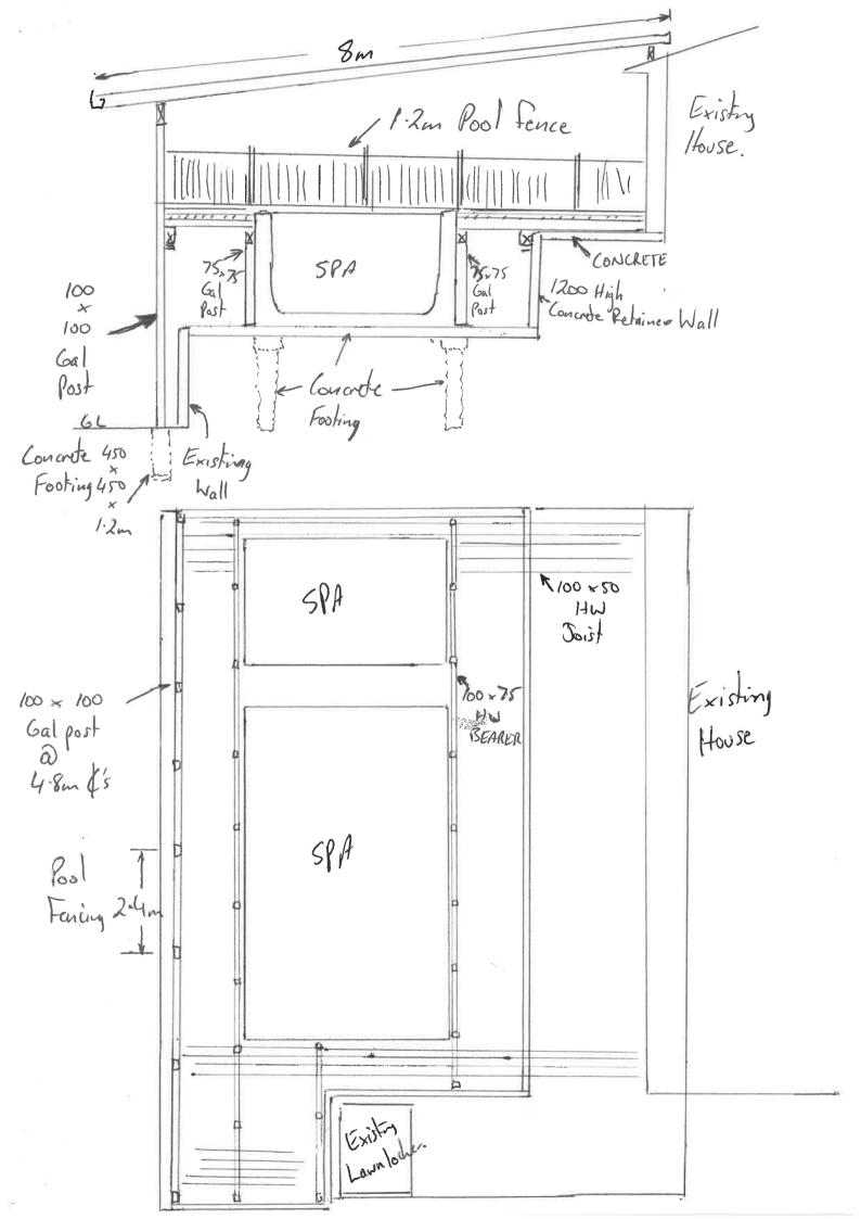
Concerte Slab + Footings as per engineering. SPB. Welded to port 450 × 460 × 1.2m Concrete Footing \$ 100 × 75 BEAKER . Thun + Run Bell, Aun 100 mm x 100 mm 100 x 50 Jeist
