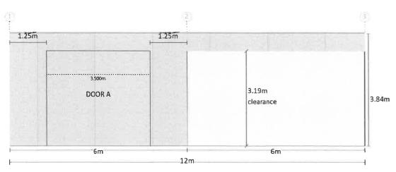
Measurements are from the outside of end girts (end bays) and/or centre of columns (mid bays) to inside of component opening size.
