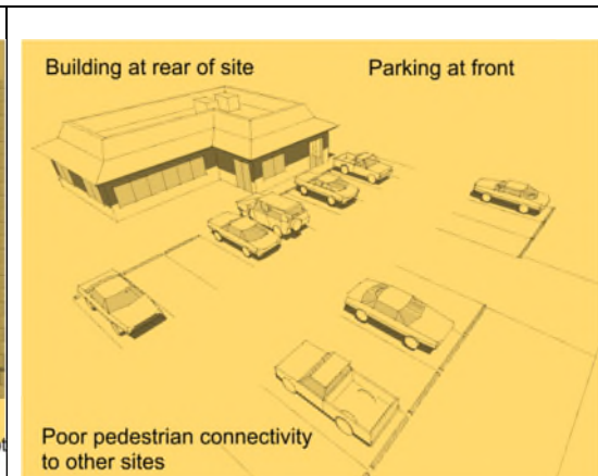
Figure SC6.7.7—Unacceptable site layout on designated commercial frontage
